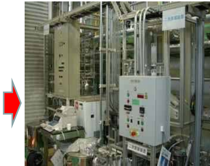
Second distillation (90%v/v) & dehydration (99.5%v/v)
