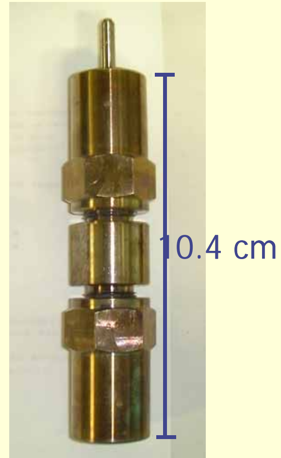
Microtube reactor (10.5 ml)
