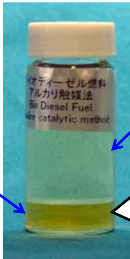
Product Obtained by Alkaline Catalyst Method
