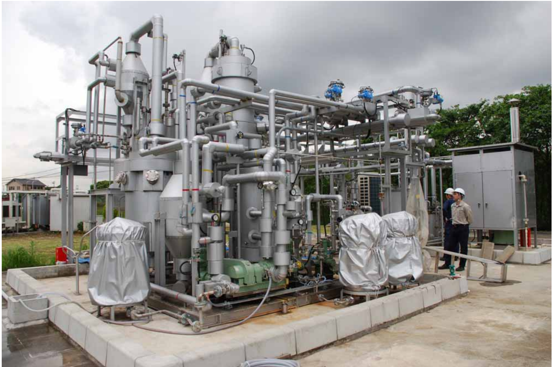
Demonstration Plant for Superheated Methanol Vapor Bubble Method (Designed Productivity: 400 L/d)
