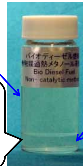
Product Obtained by Superheated Methanol Vapor Method
