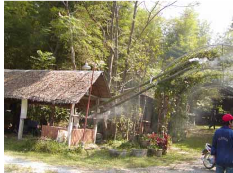
Woody biomass is mildly burned to collect wood vinegar only.
